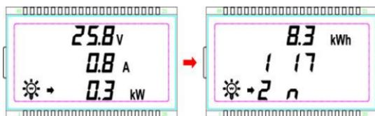
Display: Voltage/Current/Power/ Consumed energy/Load working mode-Timer1/ Load working mode-Timer2
