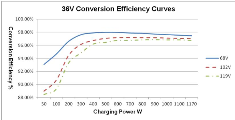
4. Solar Module MPP Voltage(68V, 102V, 119V) / Nominal System Voltage(48V)
