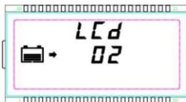
**NOTE:** The LCD cycle default time is 2s, the setting time range is 0~20s.
